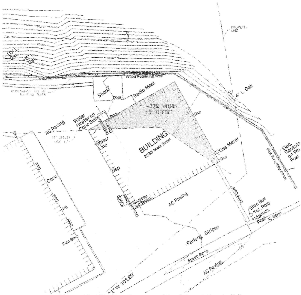
Figure 12. 15' offset from toe of bank to existing building.
